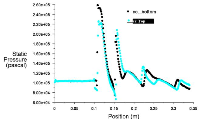
Figure 7 static pressure variations in top & bottom wall
