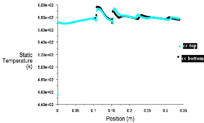
Figure 14 Static Temperature variations in top & bottom wall
