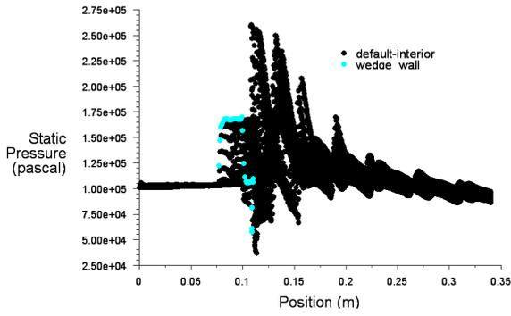
Figure 8 static pressure variations in interior and wedge wall
