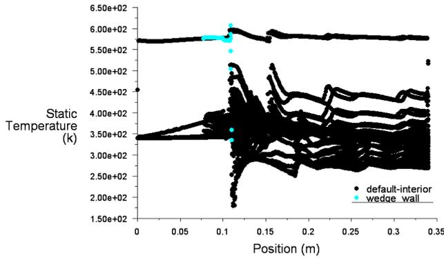
Figure 15 Static Temperature variations in interior and wedge wall
