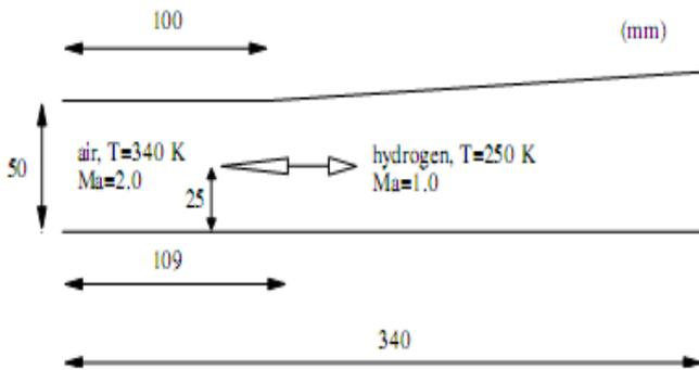
Figure 1 Schematic of the supersonic combustion chamber.
