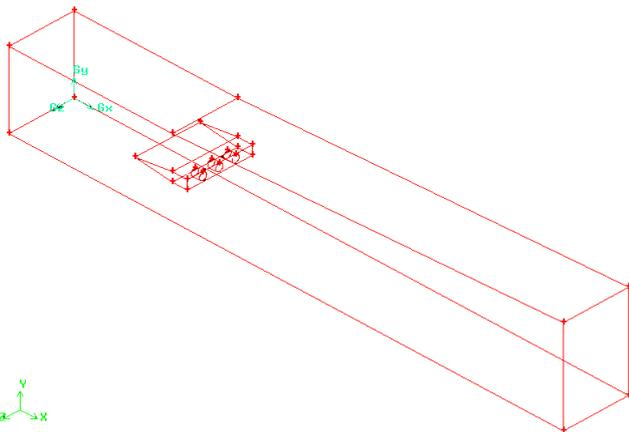
Figure- 2, 3D gambit modelling of DLR Scramjet Combustion Chamber and strut injector
