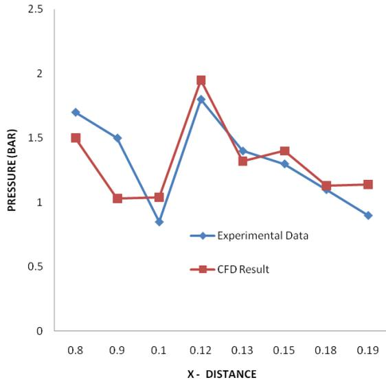
Figure 9 static pressure variations in bottom wall comparison with experimental data
