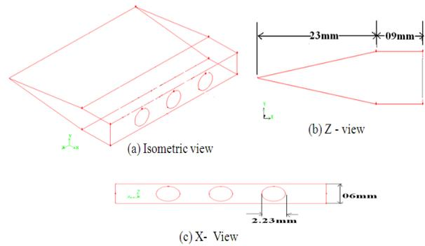
Figure- 3, 3D wedge shaped strut injector
