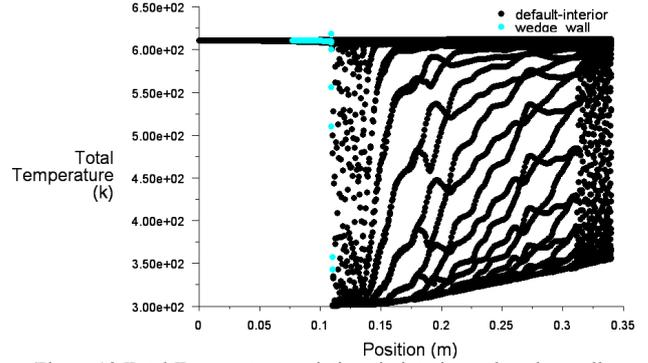
Figure 18 Total Temperature variations in interior and wedge wall
