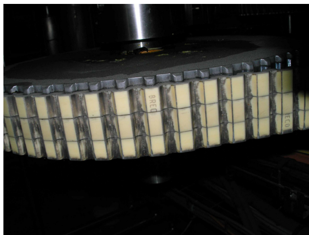
Fig.1. Drive in bottle filling machine with “special made” double sided timing belt
