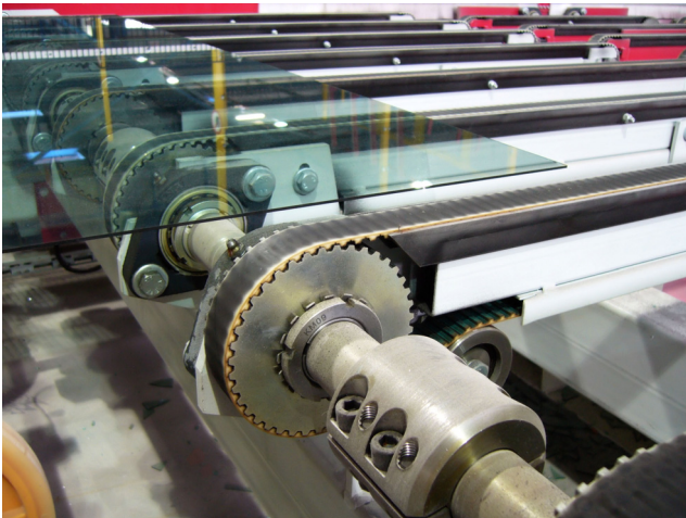
Fig.3. Parallel conveyor for glass plate cutting
