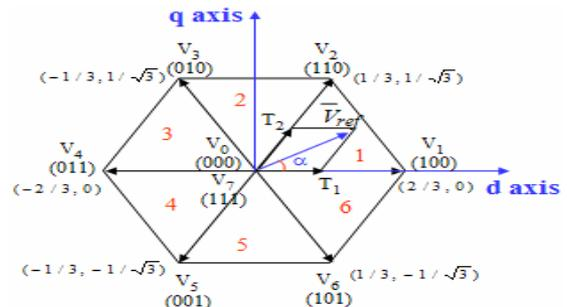
Fig 5. Basic switching vectors and sectors
