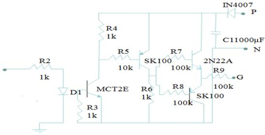
Fig 8.Driver circuit
