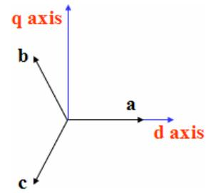
Fig 4: The relationship of abc reference frame and stationary dq reference frame.
