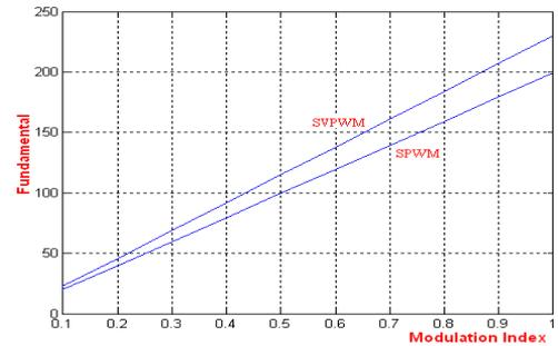
Fig 15.Fundamental Voltage Comparison of SVPWM & SPWM
