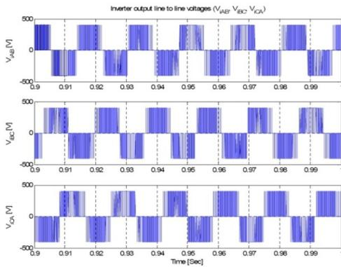
Fig 10. Simulation results of inverter output line to line voltages
