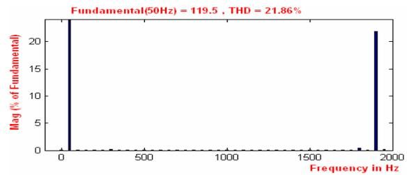
Fig 13. FFT Analysis of Output Voltage (SVPWM)
