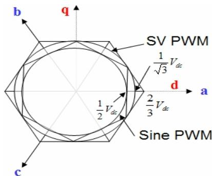
Fig 3: Locus comparison of maximum linear control voltage in Sine PWM and SVPWM.
