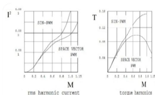
Fig 16. Harmonic Comparison of SVPWM & SPWM
