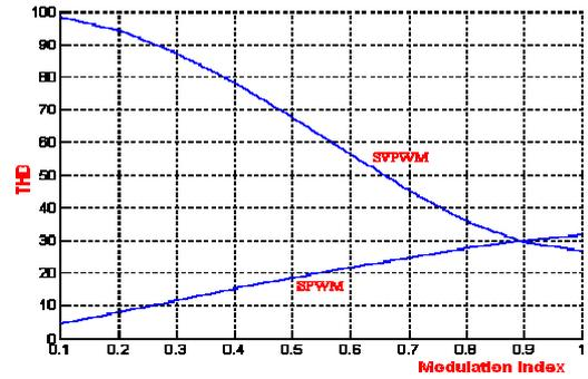
Fig 14. Fundamental & THD Vs Modulation Index (m)
