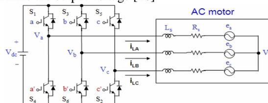
There are eight possible combinations of on and off patterns for the three upper power switches. The on and off states of the lower power devices are opposite to the upper one and so are easily determined once the states of the upper power transistors are determined. According to equations and,
