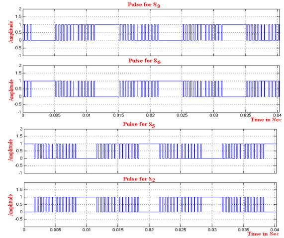
Fig 12. Triggering SVPWM pulses for the VSI circuit
