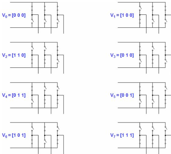
Space Vector PWM (SVPWM) refers to a special switching sequence of the upper three power transistors of a three-phase power inverter. It has been shown to generate less harmonic distortion in the output voltages and currents applied to the phases of an AC motor and to provide more efficient use of supply voltage compared with sinusoidal modulation technique as shown in Figure 5 [28]
