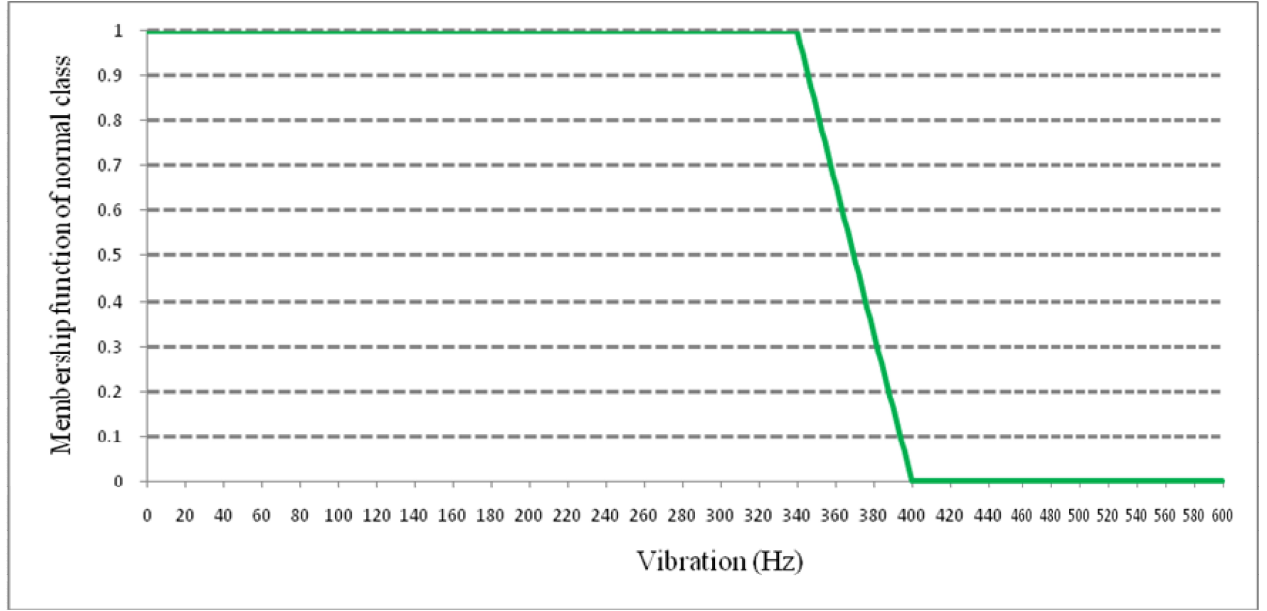
Fig. 2 Exponential membership function for vibration signals of a rotary shaft
