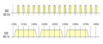
Fig. 1 Channel allocations of IEEE 802.11b and IEEE 802.15.4 technologies
