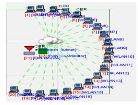
Fig .12 Circular topology Simulation Model between IEEE 802.15.4 and IEEE 802.11b
