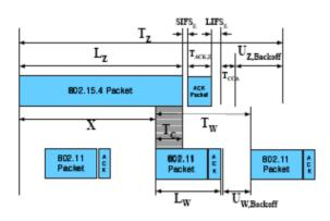
Fig.4 .Interference model between IEEE 802.15.4 and IEEE 802.11b
