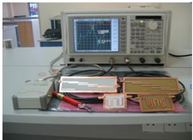
Fig. 8. Testing process using Advantest R3767CG Network Analyzer.
