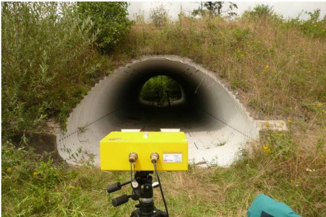
Fig. 2. View of the culvert during experimental tests using the radar.
