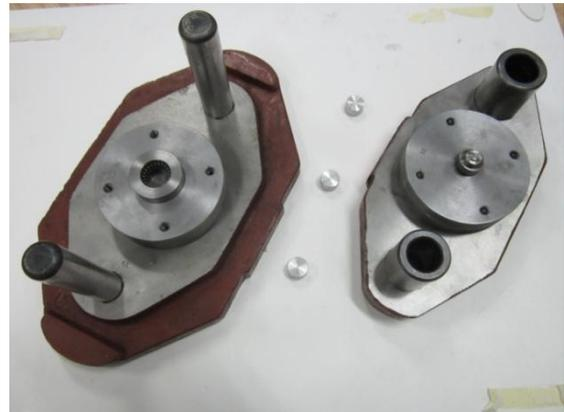
Fig. 5. Die and formed bevel gear
