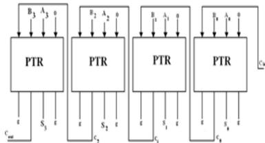
Fig. 13 4-bit reversible parallel adder using PTR gate
