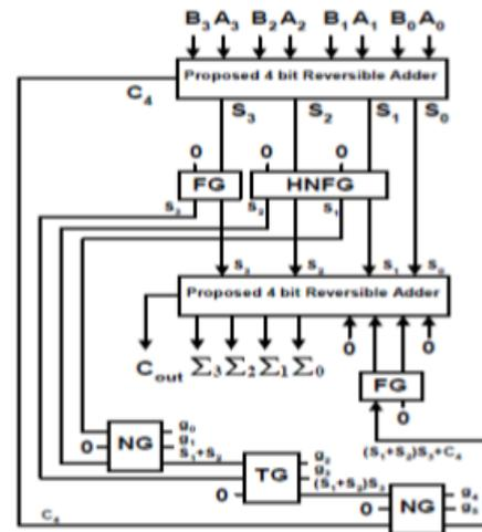
Fig. 4 Block diagram of reversible BCD adder [12]
