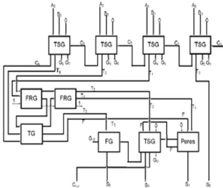
Fig. 6 Block diagram of reversible BCD adder [8]
