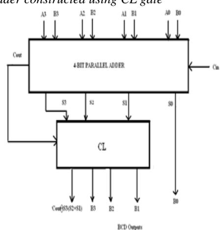
Fig. 11 BCD adder using CLgate
