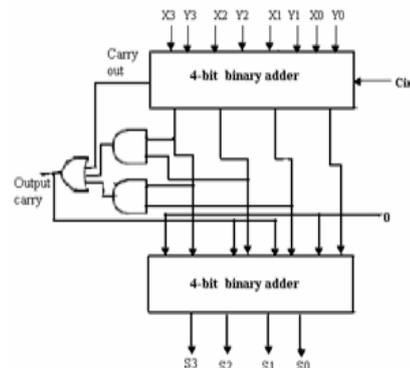
Fig. 1 Block diagram of conventional 4-bit BCD adder
