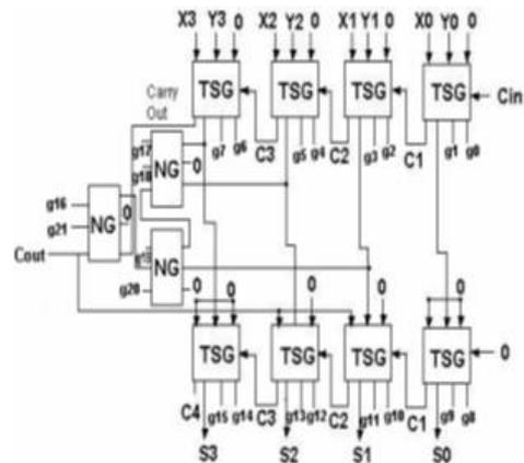
Fig. 5 Block diagram of reversible BCD adder [19]
