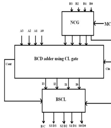
Fig. 15 BCD adder /subtractor
