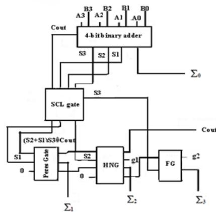
Fig. 7 Block diagram of reversible BCD adder [5]
