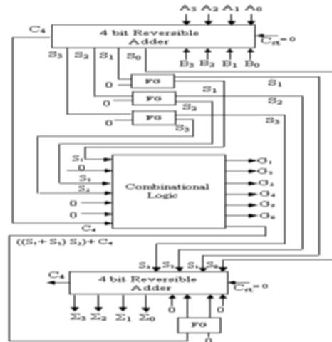
Fig. 3 Block diagram of reversible BCD adder [6]
