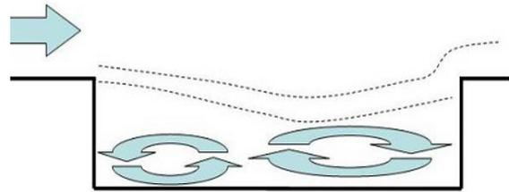
Figure 1: Rectangular cavity flame holder
