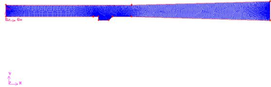
Figure 3. GAMBIT profile of wall injector (with cavity) with L/D ratio=5
