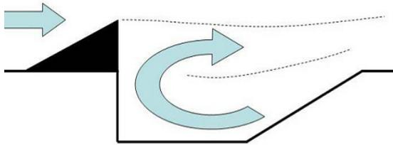
Figure 2. Cavity flame holder with inclined downstream ramp and leading edge pylon (on centerline)
